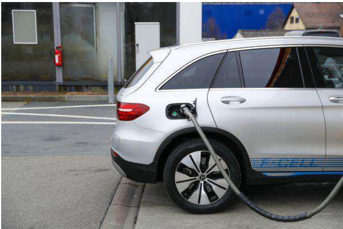
A car takes hydrogen fuel at a Royal Dutch Shell filling station in Germany.
